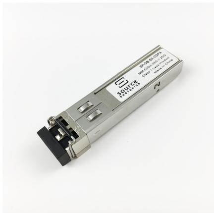
Source Photonics 1000BASE-SX 1.25Gbps 850nm VCSEL MMF 500m Módulo transceptor SFP
