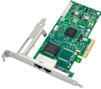
Adaptador de servidor Intel I340 Gigabit Dual RJ45 Port Ethernet, 2 puertos, RJ45, 10/100/1000, PCIe, 82580
