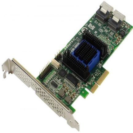
Adaptec ASR-6805E 2270900-R 6 Gb/s PCIe Gen2 x4 8 puertos Int. SAS/SATA Controlador RAID
